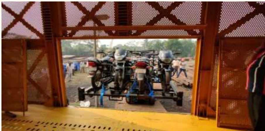
Two - wheelers loading from side door
