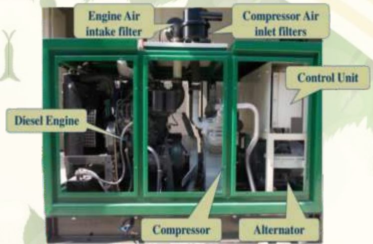
Auxiliary Power Unit
