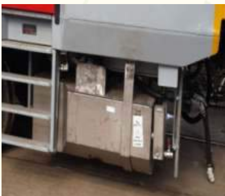
Bio-toilets fitted in Stainless Steel Bodied LHB Coaches
