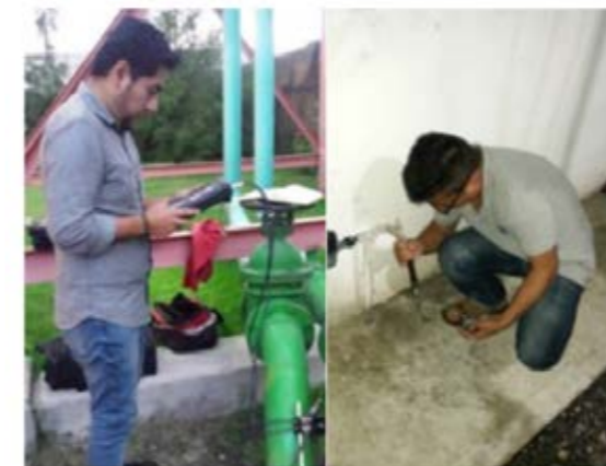
Figure 35: Use of smart water technology to measure water flow in one of the cities addressed by PADHPOT, UNAM. Source: Rocha Guzmán 2013
