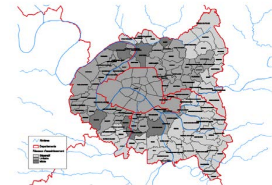
Figure 11. Typology of sewage collection inside SIAAP's administrative boundaries: Light grey: separate system, medium grey: combined system and dark grey for mixed system
