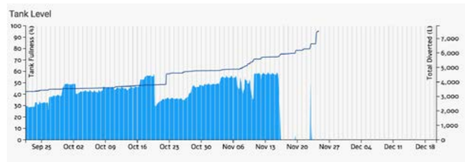
Figure 15. Rainfall-collection, tank-level, and water-use/drainage metrics for House 1 (September 20 – November 16) [Showing collection when filters are not clean]
