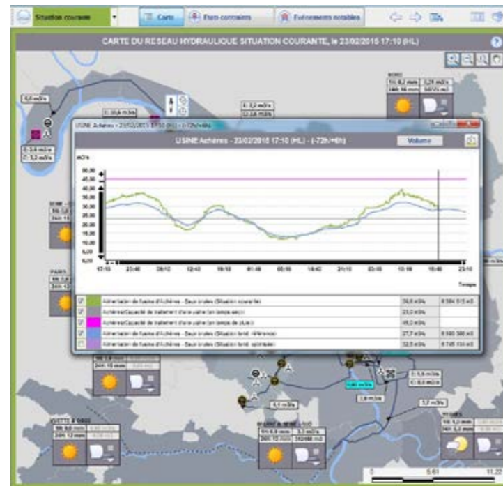
Figure 30. Screen shot of flow prediction at Seine-Aval WWTP planned (green curve: measurement, blue curve: model)
