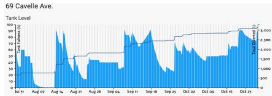
Figure 12. Rainfall collection, tank-level and water-use/drainage metrics for Household 4 (August 28 – October 28)
