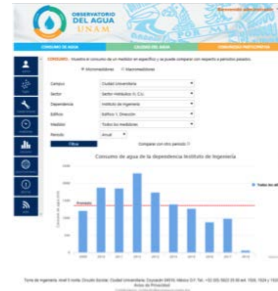
Figure 30. Graph showing annual water consumption of one of the buildings of the Institute of Engineering, UNAM.
