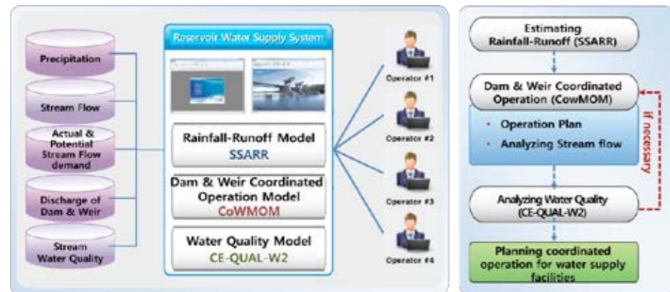
Figure 18. Reservoir Water Supply System (RWSS) (Source : K-water)
