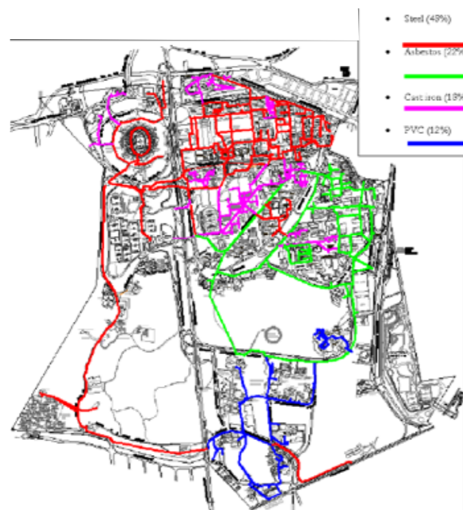
Figure 5. Digitalized water supply network of the University City of UNAM. Pipeline colours correspond to different materials: steel, asbestos, cast iron, and PVC. Source: PUMAGUA, 2012
