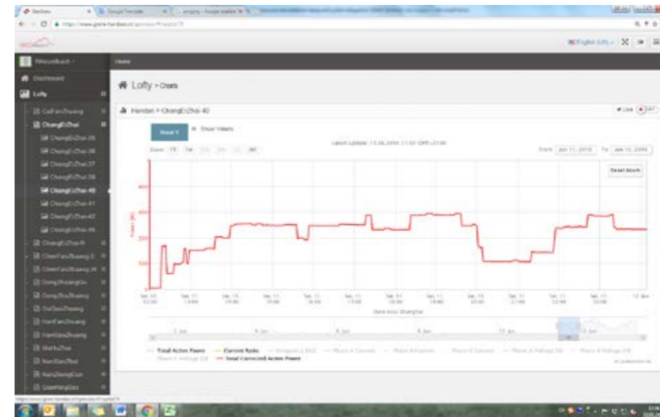
Figure 9. An example of real-time data display, received from the ChangErZhai-40 station. Users can pick any sensor and view data from a certain time period. The chart illustrates the real-time power of pumping well transformers, which reflects the current working condition of pumping wells.
