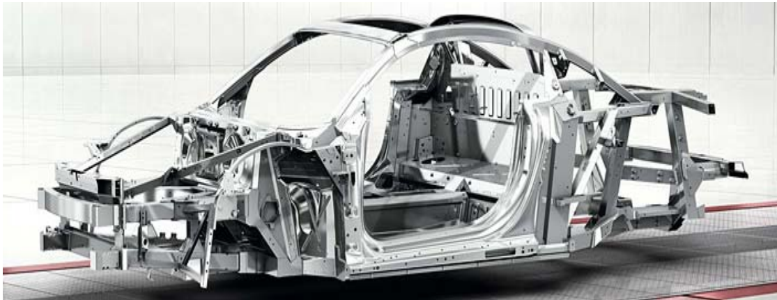
Figure 25: The all-aluminum Audi Space Frame (ASF) system, for illustration purpose only, courtesy of AudiUSA.com.
