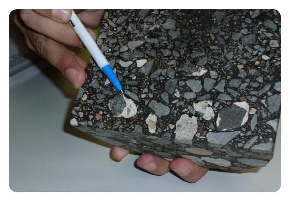
65% Recycled asphalt showing recycled material aggregate.
