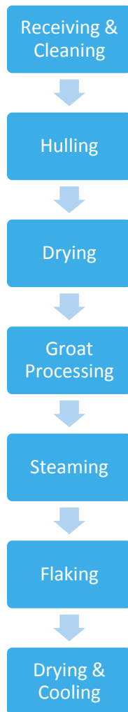
Figure 7: Traditional oat cereal production process (based on Caldwell et al., 2000b)
