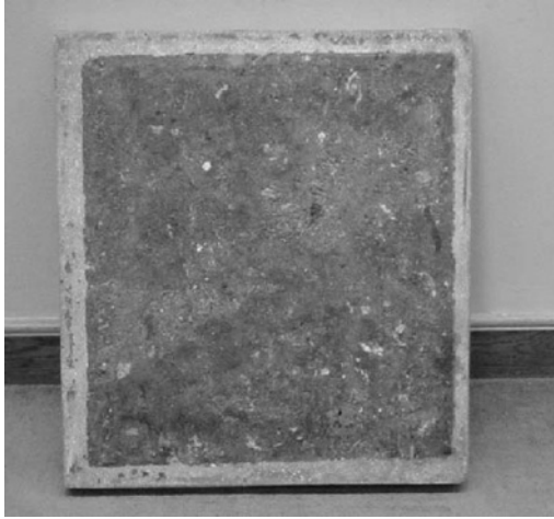
FIGURE 6.11 Table topping from rejects
