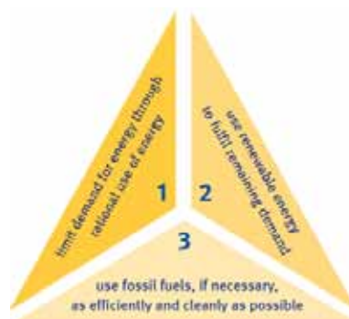
Figure 2 - 1 The Trias Energetica is a logical concept to inform our use of energy.
