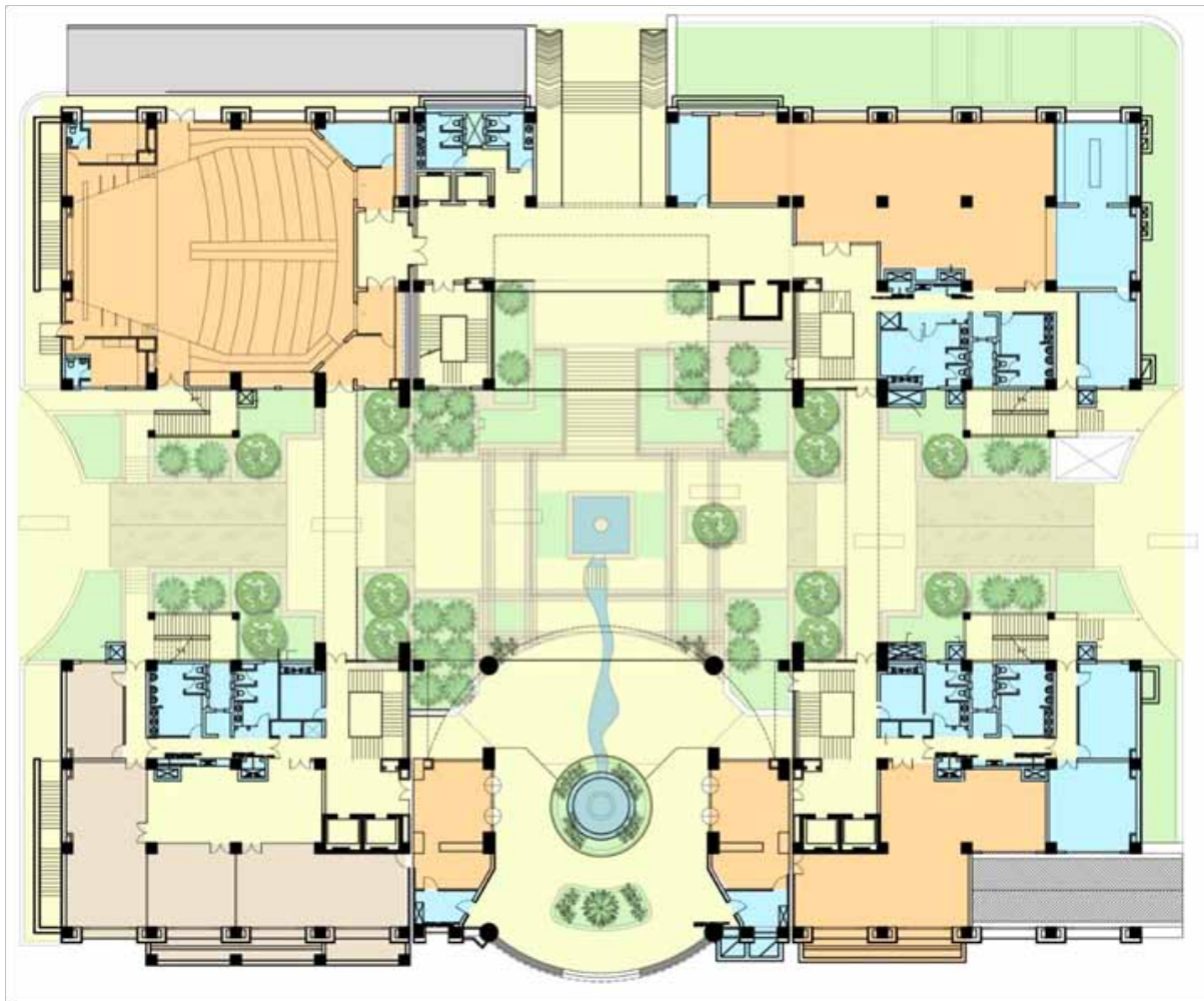
Figure 19.3 Final plan developed with emphasis to the north–south axis and the central courtyard
