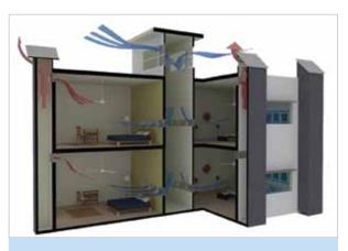
Figure 5 Downdraft cooling system
