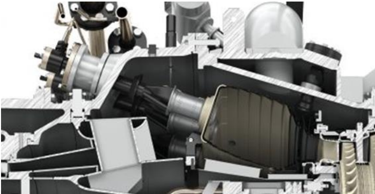
Figure 11: 3rd generation DLE combustion system
