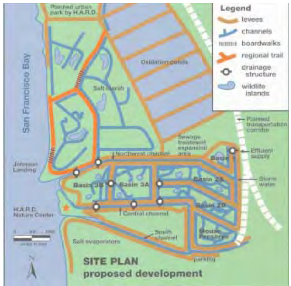
Schematic of the Hayward Shorline Marsh Expansion Project.
