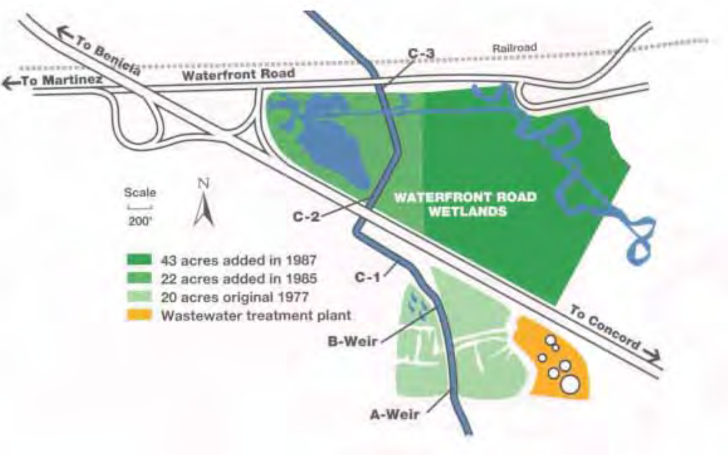
Schematic of the Mt. View Sanitary District marsh creation project.
