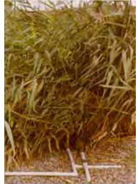
Intensive studies carried out for over 5 years at Santee, CA, evaluated the performance of constructed wetlands experimental units planted with reeds, cattails, and bulrush..
