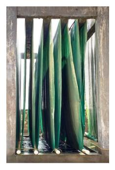
Figure 1: Photo plate of Net Evaporator at JITPPL at Jaipur for R O Rejects of Textile CETP
