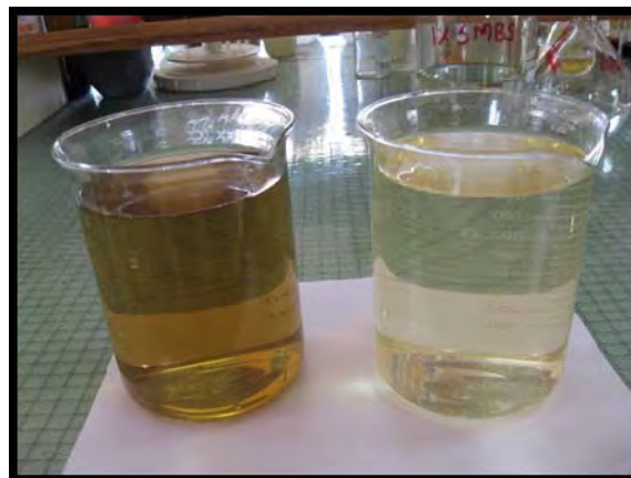
R.O reject – before treatment
