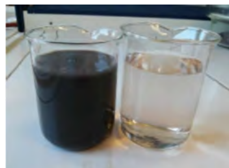
MBR inlet and outlet textile effluent
