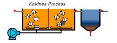
MBBR Process (standalone no RAS; can be multiple reactors depending on BOD, Nitrify, De-nitrify, TSS loading)
