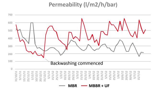
Higher permeability and longer cleaning intervals (4 times less chemical used) for MBBR + UF compared to MBR
