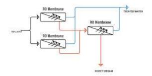
**Figure 1**: Schematic of a Reverse Osmosis Process Used in Zero Liquid Discharge.
