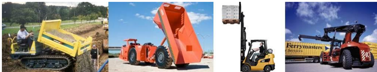
Figure 1: Earth-moving and transportation machines (left to right): Amman Yanmar small dumper C30R-1 ( http://us.yanmar.com ), Sandvik TH320 underground truck ( http://mediabase.sandvik.com ), Caterpillar forklift GC20-33N ( http://www.rocla.com ), Kalmarr DRF Reach Stacker ( http://www.kalmarind.com ).
