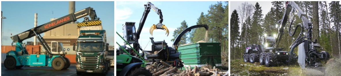
Figure 9: Commercial high power, hybrid mobile machines: Konecranes SMV 4531 TB5 HLT hybrid reach stacker ( http://www.konecranes.com ), KESLA C860 Hybrid wood chipper ( http://www.kesla.com ), and Logset 12H GTE Hybrid forest harvester ( http://www.logset.com ).
