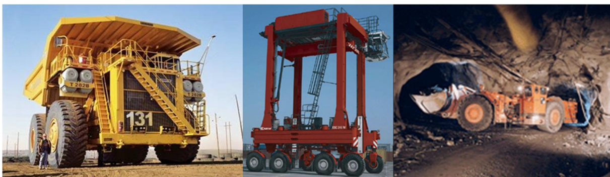
Figure 8: Commercial high power, electric driven work machines: Liebherr T282B Dump Truck 2.7 MW ( http://www.liebherr.com ), Kalmar ESW Straddle Carrier 400 kW ( http://www.klamarind.com ), and Sandvik long haul dump Toro 2500E 315 kW ( http://mediabase.sandvik.com ).
