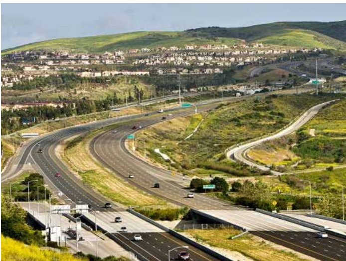
Low density increases VMT: This development in Orange County, CA is not person-scaled, but car-scaled. Low-density development encourages a car-centric lifestyle, making it trip distances longer and increasing VMT. Photo credit: David Eppstein / Wikimedia Commons
