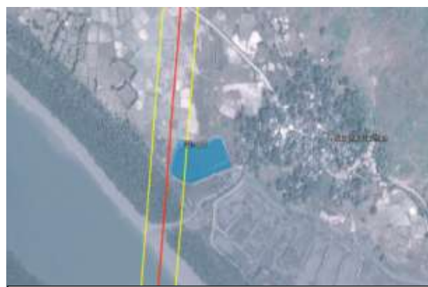
Chainage – 32+000 Total area of the Pond: 15,336.23 Sq.m Affected area of the Pond: 3,557.39 Sq. m
