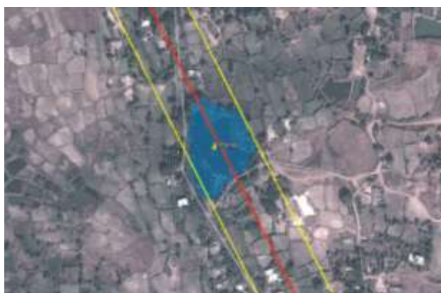
Chainage – 27+850 Total area of the Pond: 8,622.50 Sq.m Affected area of the Pond: 8,216.79 Sq. m
