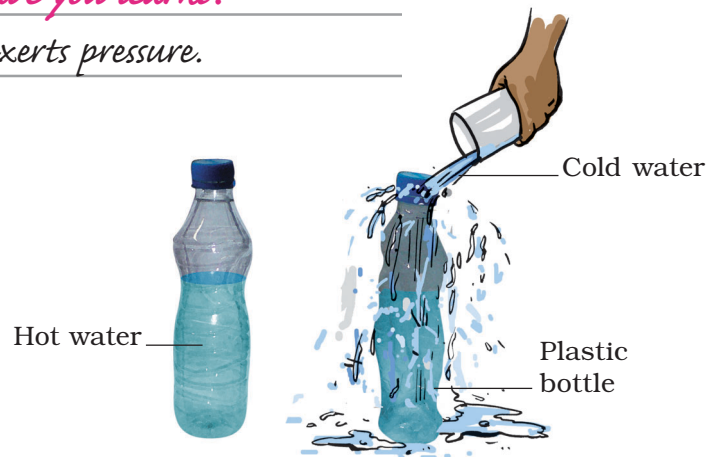
Fig.7.5.2 Bottle with hot water deformed when cooled
