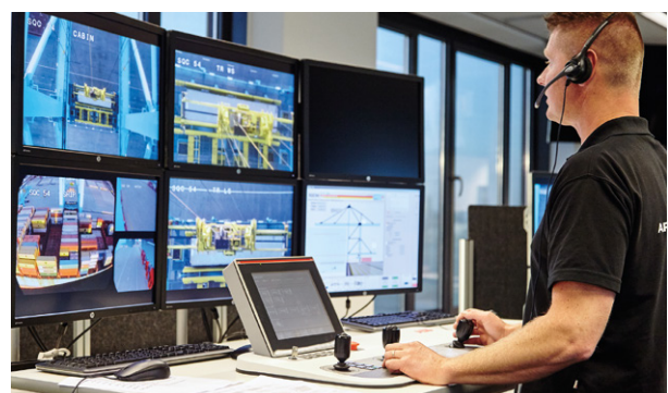
Fig 9: Remote control station of quay crane
