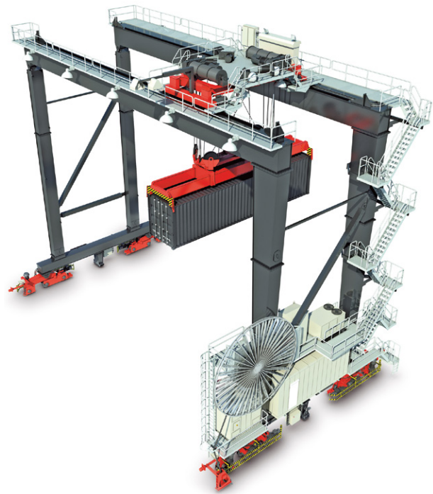
Fig. 2: A typical ARMG design where containers are moved along the gantry direction and transfer vehicles are served at block ends
