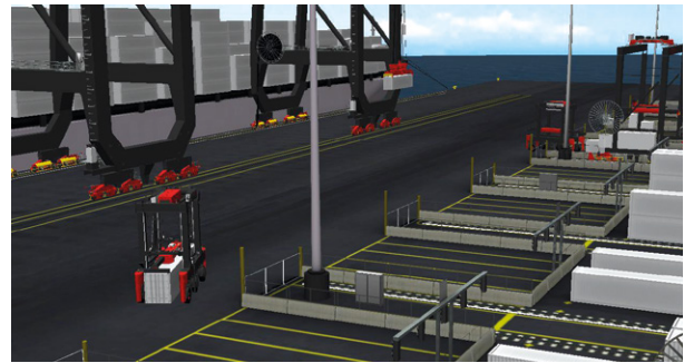
Fig 5: Waterside horizontal transport with shuttle carriers in the end-loading ARMG layout
