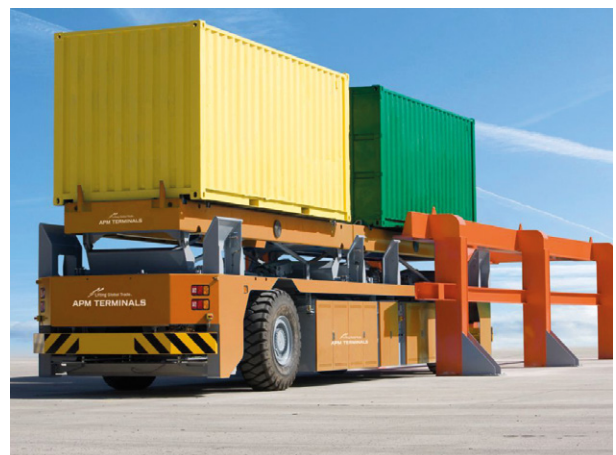
Fig 7: Elevated rack for “lift” platform vehicle
