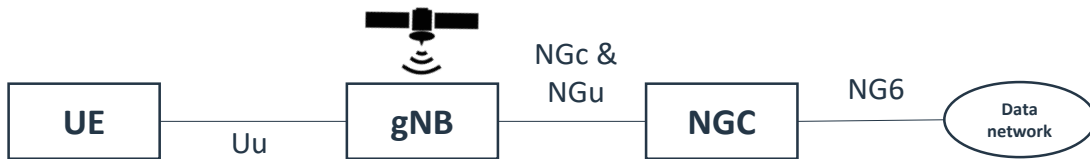
Figure 5.2. NTN Featuring an Access Network Serving UEs and Based on a Satellite/Aerial with gNB on Board. 46
