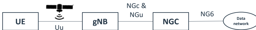
Figure 5.1. NTN Featuring an Access Network Serving UEs and Based on a Satellite/Aerial with Bent Pipe Payload and gNB on the Ground (Satellite Hub or Gateway Level). 45
