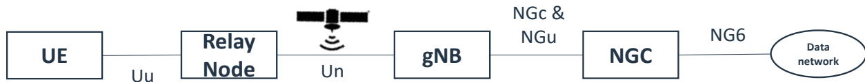
Figure 5.3. NTN Featuring an Access Network Serving Relay Nodes and Based on a Satellite/Aerial with Bent Pipe Payload.
