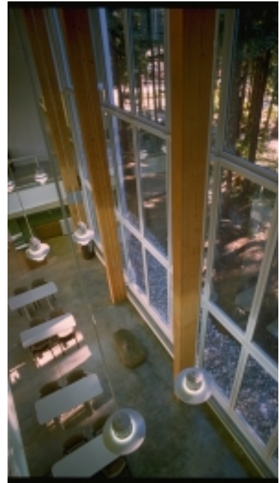
Daylight and occupancy sensors in the CK Choi Building, UBC reduce the use of artificial lighting. The lighting load is 0.9 w / sq. ft.
