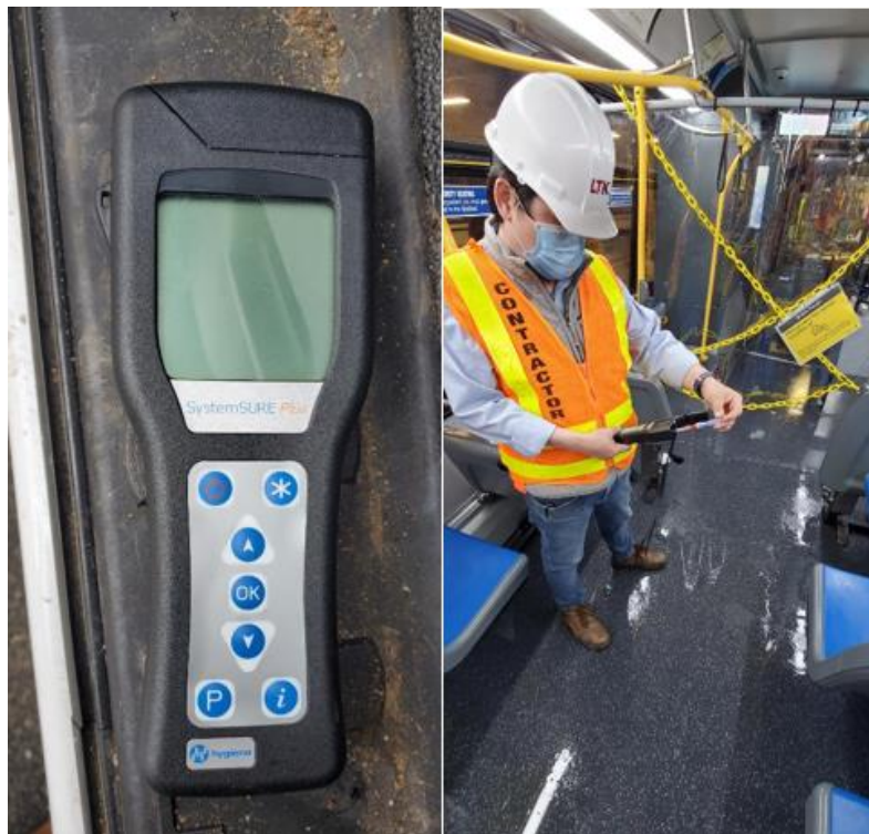
Example ATP Unit (Left) and Test Being Performed on a Bus (Right)
