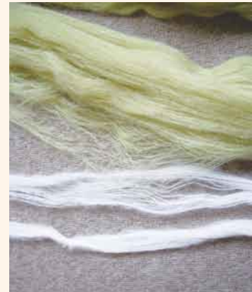
Fuga 1/44mm mohair yarn developed by Sato Seni, which is much finer than prior yarns
