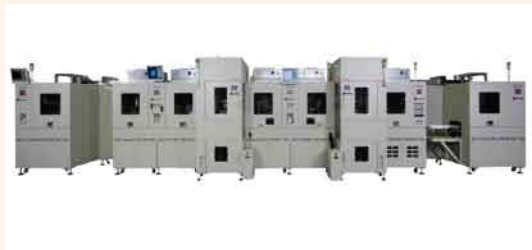
The world's first fully automated FOB line, developed by Ohashi Engineering
