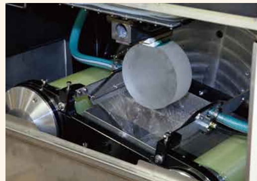
Sapphire cutting using a Takatori Corporation multi-wire saw.
