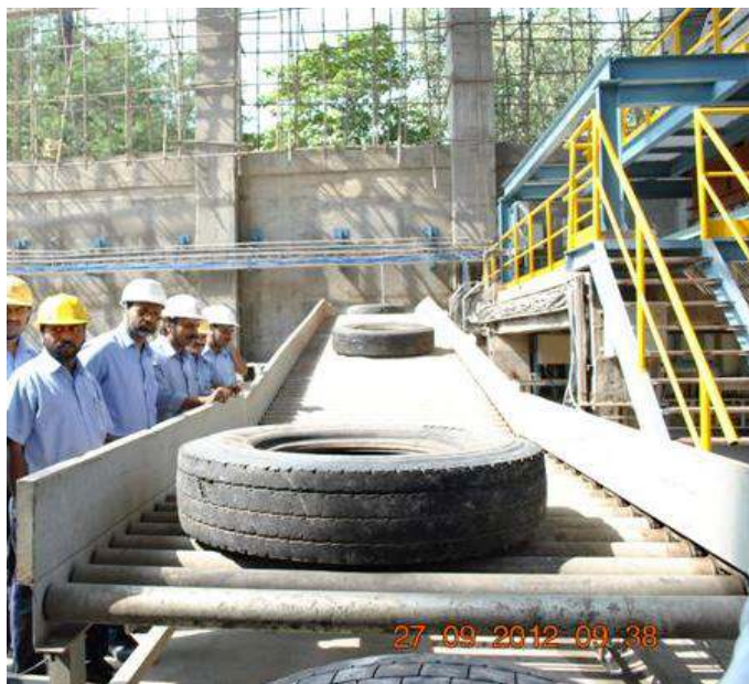
Fig: Whole tyre feeding system
