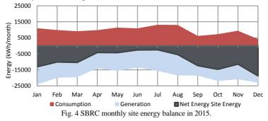
The total generation for the year was 225 MWh – an average of 617 kWh per day, and above the design target. The total consumption was 115 MWh, averaging 316 kWh per day. This translates to an energy intensity of 44.3 kWh/m<sup>2</sup>/year for 2015.
