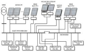
Fig. 2 Line diagram of SBRC electrical distribution system.
