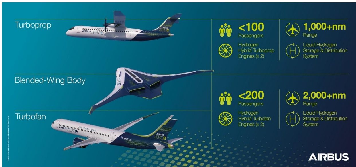
Figure 15: Airbus ZEROe aircraft concepts towards a hydrogen-fuelled aircraft that commercially enters into service in 2035 (Airbus, 2020).
