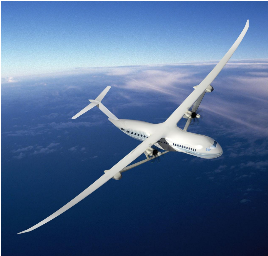
Figure 22: Artist impression of the Boeing SUGAR Volt concept, utilising a truss-braced high aspect ratio wing (NASA, 2010; Bradley & Droney, 2011; Bradley & Droney, 2015; Wall & Meyer, 2017)
