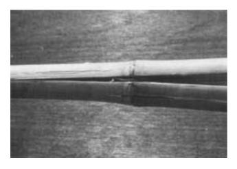
Fig9: The punch fracture behavior of bamboo
