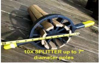
Fig10: Bamboo Splitting
