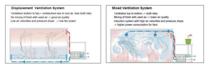
By displacement ventilation system, the air is supplied near the floor to a distance of 10-15m and exhausted near the ceiling. This requires lower air volume movement rates, leading to lower fresh air intake rates and less electricity required to drive the fan for both air exhaust and supply.
