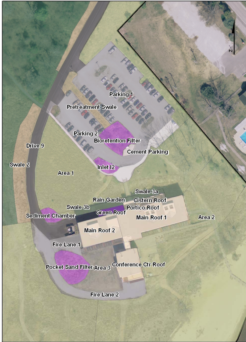
Figure E-6 Watersheds used in the Merrill Center 'existing condition' P8 model. The labeled watersheds are included in the Limit of Disturbance (LOD) models
