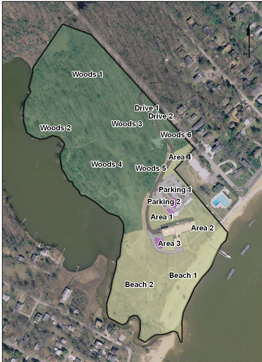
Figure E-5 Watersheds used in the Merrill Center 'existing condition' P8 model. Many of these areas are outside of the limit of disturbance. For watersheds near the building, please see Figure E-6
